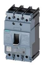
circuit breaker 3VA5 UL frame 125 breaking capacity class S 25kA @ 480 V 3-pole, line protection TM230, FTAM, In=15A overload protection Ir=15A fixed short-circuit protection Ii=10...20 x In cable connection on both sides
