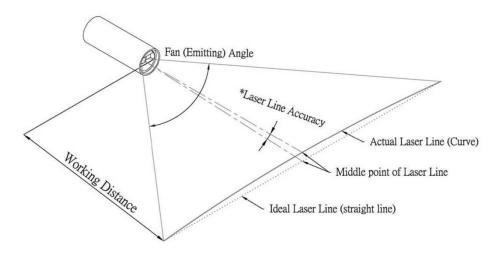
\*Laser Line Accuracy The error angle between Ideal and Actual Laser Line at middle point. For VLM-635/650-27 Series, Laser line accuracy < 40" (Arc Second) =  $\frac{40}{3600}$ ° (Degree) For VLM-635/650-37 Series, Laser line accuracy < 20" (Arc Second) =  $\frac{20}{3600}$ ° (Degree) For VLM-532-46 Series, Laser line accuracy < 20" (Arc Second) =  $\frac{20}{3600}$ ° (Degree)
