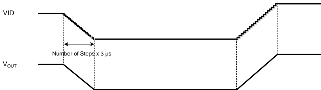
Figure 5-4. DVS Timing Diagram I (BUCKx_DECAY = 0)
