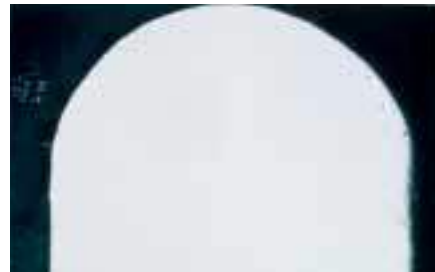
Cross sectional view of PANDUIT® tie body. (Photo micrograph shown is magnified 150X).
