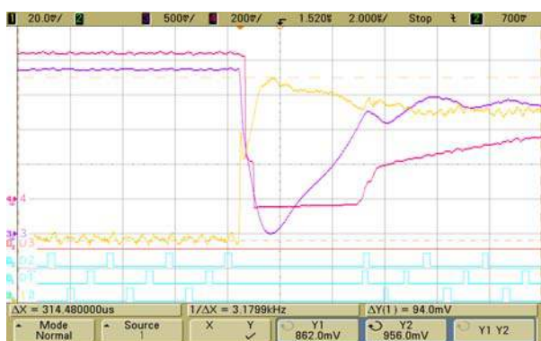
Figure 10. Typical Transient Response for Design Example Load Release 1-Vo, 3-COMP, 4-TRDET, D0~D2-PWM1~3
