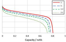
Charge : CC-CV 1C, 2.8V, cut-off 0.05C at 25°C
