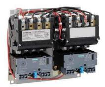
2-speed 3-phase motor starter Size 2 Two separate windings Constant or variable torque Solid-state overload relays Low SPD OLR range 13-52a High SPD OLR range 13-52a 110-120/220-240VAC 60HZ coil Enclosure NEMA type (open) No enclosure
