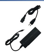
Use only the power cord provided with the unit (4 ft - 1.2m) or equivalent UL approved type SPT-2, SVT, or SJT 18/3 AWG 100-240 VAC, 1 Amp  $60^{\circ}$ C:
