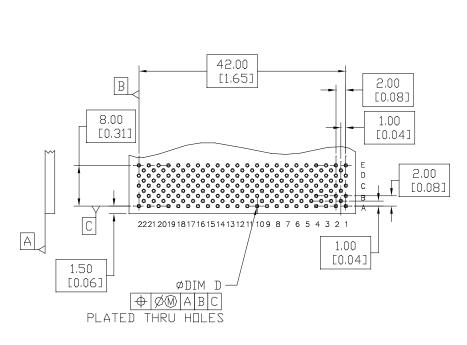
Recommended PCB hole mounting pattern for coaxial, Column differential and stripline applications..
