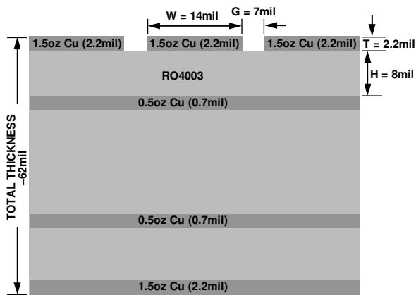
Figure 23. Evaluation Board Cross Sectional View
