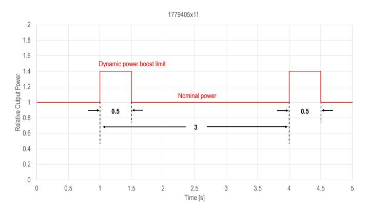
**Note:** The overload current of 150%  $I_{OUT}$  can be supplied for maximum 0.5s and requires a 3s recovery time till next overload event.
