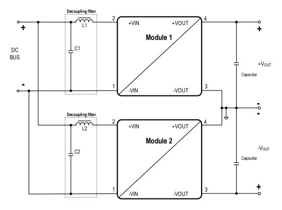
For using long supply lines or different line length for each 1779405X11 it is recommended to decouple each power module with an additional LC- filter. The decoupling LC-filter is also recommended if the supplying dc bus has a high impedance so that high voltage swings at the input of each power module could be present. As initial values, the EMI filter shown for every part number can be used. See also "Primary side parallel connection".
