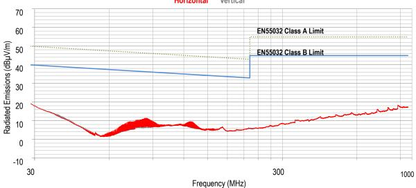
Conducted Emissions 1779405211  $V_{\text{IN}} = 12\text{V, V}_{\text{OUT}} = 5\text{V, I}_{\text{LOAD}} = 0.4\text{A with input filter}$   $C_F$  and  $C_{\text{IN}} = 4.7\mu\text{F}$  (885012209013),  $L_F = 6.8\mu\text{H}$  (744773068),  $C_{\text{OUT}} = 10\mu\text{F}$  (885012209014),  $C_Y = 1\text{nF}$  (885342210001)
