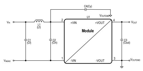
For optimal EMI performance, one filter capacitor, C1, one filter inductor, L1, one input capacitor, C2, one output capacitor, C3 and one Y-Cap, C4 are recommended. For optimal electrical performance, one input capacitor C2 and one output capacitor C3 are recommended.
