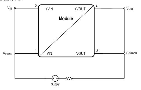
Parameters Supply Device: Current limit set 1mA, test voltage 1500 VDC, test time 60s.
