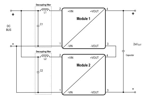
In case of using long supply lines or different line length for each 1779405X11 it is recommended to decouple each power module with an additional LC filter. The decoupling LC filter is also recommended if the supplying dc bus has a high impedance so that high voltage swings at the input of each power module could be present. As initial values, the EMI filter shown for every part number can be used. See also "Primary side parallel connection".
