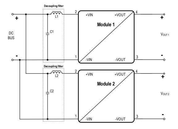
As a starting point for the decoupling filters, use the values of the reference filters - see also "RADIATED AND CONDUCTED EMISSIONS (WITH EMI INPUT FILTER))". The final appropriate filter for the application has then to be evaluated under operation in the target application by checking e.g. the change of the input ripple voltage.
