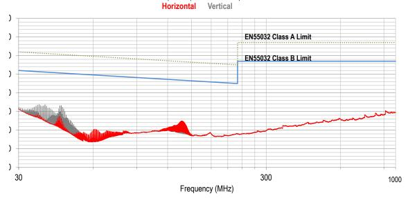
Conducted Emissions 1779405311  $V_{IN} = 24V, \ V_{OUT} = 5V, \ I_{LOAD} = 0.4A \ \text{with input filter}$   $C_F \ \text{and} \ C_{IN} = 4.7 \mu F \ (885012209048), \ L_F = 6.8 \mu H \ (744773068), \ C_{OUT} = 10 \mu F \ (885012209014), \ C_{Y} = 1 n F \ (885342210001)$
