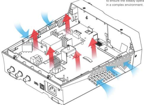
DG900 Series Function/Arbitrary Waveform Generator
