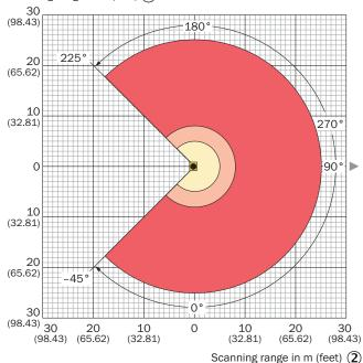
Range for **not safety-related** detection at > 90% remission: 0.05 m (0.17 feet) to max. 25 m (82.02 feet) (3)
