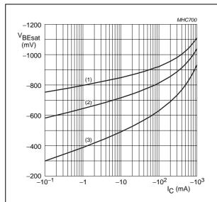
Transistor TR1;  $I_C/I_B = 20$ .
