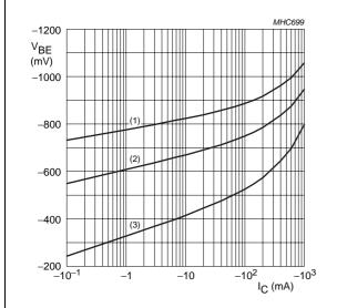
Transistor TR1;  $V_{CE} = -2 V$ .
