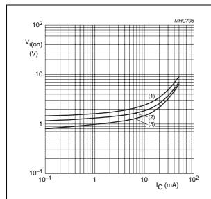
Transistor TR2;  $V_{CE} = 0.3 \text{ V}.$
