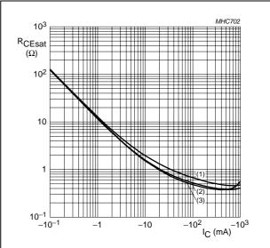
Transistor TR1;  $I_C/I_B = 20$ .
