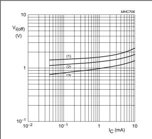
Transistor TR2;  $V_{CE} = 5 V$ .
