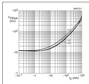
Transistor TR1;  $I_C/I_B = 20$ .
