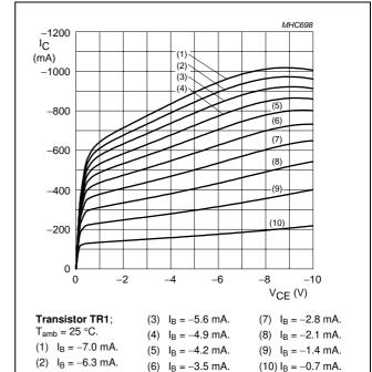
Fig.3 Collector current as a function of collector-emitter voltage; typical values.
