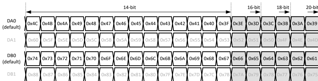
Figure 8-44. 1-wire output bit mapping
