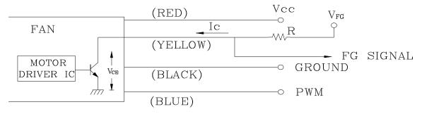
CAUTION: THE LEAD WIRE OF FG SIGNAL CAN NOT TOUCH THE LEAD WIRE OF POSITIVE OR NEGATIVE.
