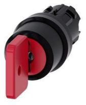
Key-operated switch O.M.R, 22 mm, round, plastic, lock number 73037, red, with 2 keys, 3 switch positions I-O-II, latching, actuating angle 2x45°, 10:30h/12h/13:30h, key removal O, with laser labeling, upper case and lower case, always upper case at beginning of line
