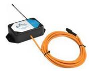
The ALTA Wireless Water Rope Sensor detects the presence of water anywhere along the surface of the rope. Sensor comes with 10' of water rope. Additional 10 ft. sections are available and can be connected up to 100 feet.
