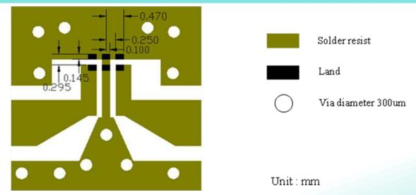
Line width should be designed to match  $50\Omega$  characteristic impedance, depending on PCB material and thickness.
