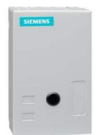
Non-reversing NEMA contactor, Size 00, Three phase full voltage, Contactor amp rating 9A, 3 wire (NO aux included), 220-240/440-480VAC 60Hz coil, Non-combination type, Enclosure NEMA type 1, Indoor general purpose use, Extra-wide enclosure
