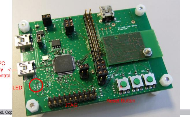
Connect with PC for power supply <and terminal control
