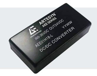
Standard features include 1,500 Vdc input/output isolation, comprehensive protection against overvoltage, overcurrent and overtemperature conditions, and remote On/Off.
