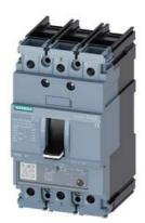
circuit breaker 3VA5 UL frame 125 breaking capacity class M 35kA @ 480 V 3-pole, line protection TM230, FTAM, In=45A overload protection Ir=45A fixed short-circuit protection Ii=5...10 x In UL489 SB (naval), 50 deg. cel. cable connection on both sides
