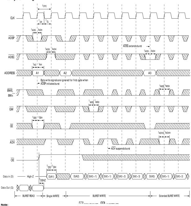
18. Full width write can be initiated by either  $\overline{\text{GW}}$  LOW; or by  $\overline{\text{GW}}$  HIGH,  $\overline{\text{BWE}}$  LOW and  $\overline{\text{BW}}_{\text{[A:D]}}$  LOW.
