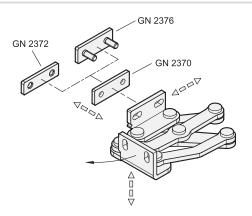
The stainless steel multiple-joint hinges can be adjusted in three planes during installation. For example, this allows adjustment for tolerances or establishing of required compressive forces for seals.
