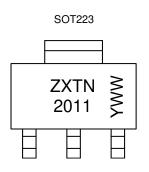
ZXTN 2011 = Product Type Marking Code YWW = Date Code Marking Y or  $\overline{Y}$  = Last Digit of Year (ex: 5= 2015) WW or  $\overline{W}W$  = Week Code (01~53)
