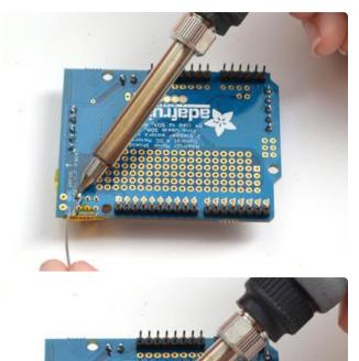
Then flip the board over and solder the 6 pins
