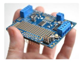
OK next up take the 2x3 pin header and place it with the short legs down into the top corner where it says SERVO 1 and SERVO 2
