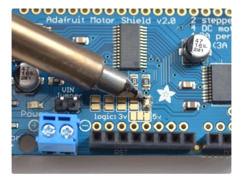
Board 0: Address = 0x60 Offset = binary 0000 (no jumpers required)
