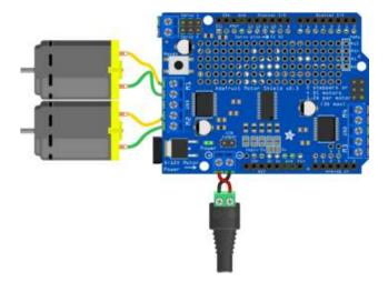
Connect the two motor wires from the first motor to the M1 terminal on the Shield.
