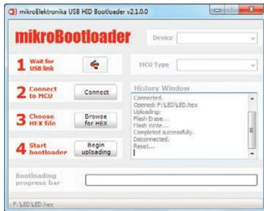
Figure 3-8: mikroBootloader ready for next job
