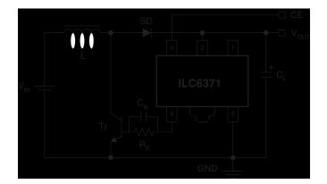
L:  $100\mu$ H SD: Schottky diode C<sub>L</sub>:  $47\mu$ F 16V (Ceramic or Tantalum Capacitor) R<sub>B</sub>:  $1k\Omega$ C<sub>B</sub>: 3300pF Tr: 2SC3279, 2SDI628G
