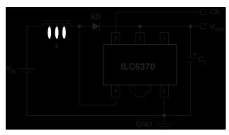
L: 100 $\mu$ H SD: Schottky diode C<sub>L</sub>: 47 $\mu$ F 16V (Ceramic or Tantalum Capacitor)
