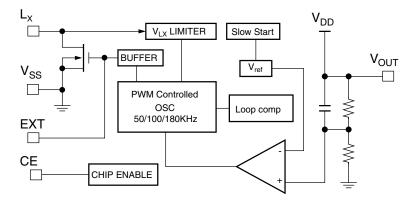
$V_{DD}$  is internally connected to the  $V_{OUT}$  pin.
