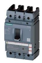
circuit breaker 3VA5 UL frame 250 breaking capacity class M 35kA @ 480 V 3-pole, line protection TM230, FTAM, In=175A overload protection Ir=175A fixed short-circuit protection Ii=5...10 x In UL 489 SB (naval), 50° C without connection
