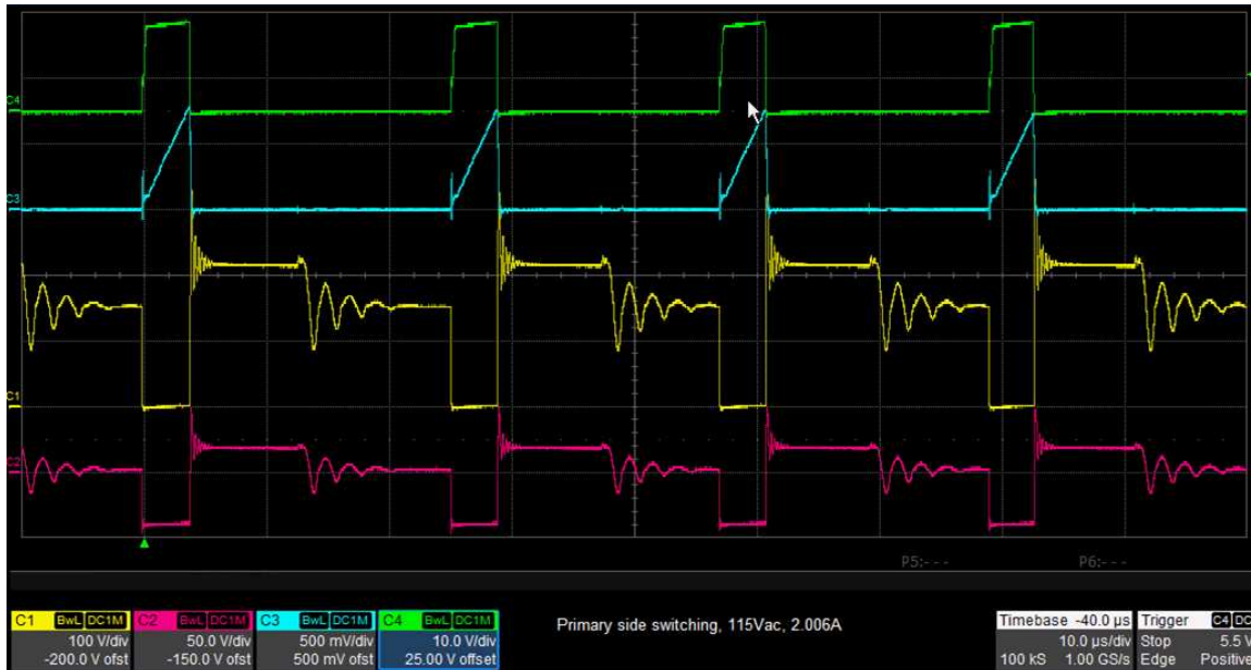
Figure 14. Primary-Side Switching Waveform
