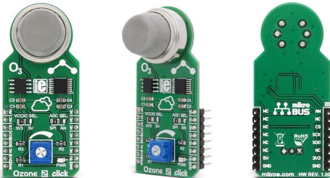
**Ozone 2** click carries an MQ131 sensor for Ozone ( $O_3$ ). The sensor outputs an analog voltage, which is converted by the onboard MCP3551 22-bit ADC converter or it is sent to the microcontroller via AN pin on the mikroBUS™, depending on the position of ADC SEL. jumper. The click is designed to run on 5V power supply. It communicates with the target microcontroller over SPI interface or AN pin on the mikroBUS™ line.
