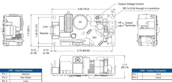
Mates with JST housing VHR-2N and JST Series SVH-21T-P1.1 crimp terminals
