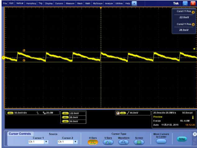
Figure 4-1 V_{in}=100V_{ac} , V=50mV/div , H=20ms/div V_{out} ripple= 50mV_{p-p} , P_{out}=0W
