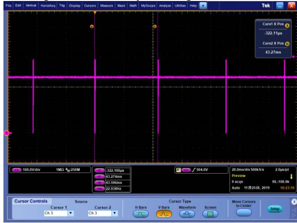
Figure 8-1 No-load, V=100V/div, H=20ms/div, Skip mode, f=22.9 kHz
