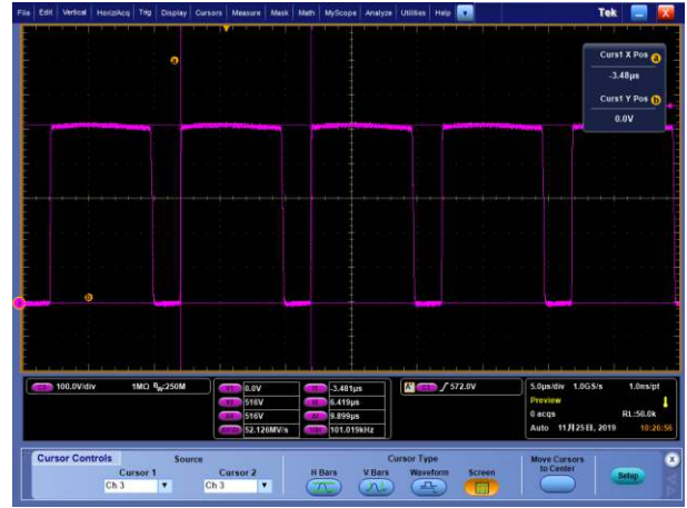
Figure 8-2 100% load, V=100V/div, H=5µs/div ACF mode. F=101 kHz, Vsw=516V
