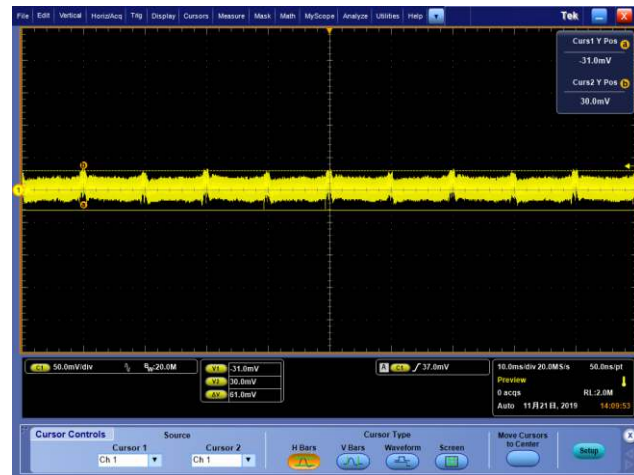
Figure 4-3 V_{in}=100V_{ac} , V=50mV/div , H=10ms/div V_{out} ripple= 61mV_{p-p} , P_{out}=102W
