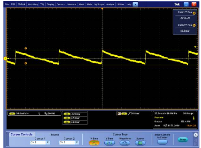
Figure 4-2 V_{in}=230V_{ac} , V=50mV/div , H=20ms/div V_{out} ripple= 74mV_{p-p} , P_{out}=0W
