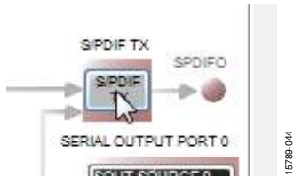
Figure 42. Configuring the S/PDIF Transmitter Routing Matrix Register
