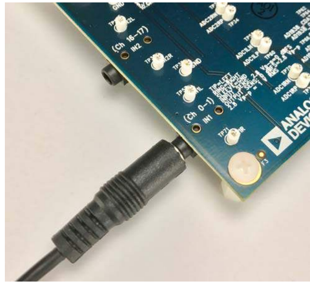
Figure 11. Analog Stereo Input Source Connection
