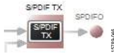
Figure 44. Confirming that the DSP Core Outputs are Routed to the S/PDIF Transmitter
