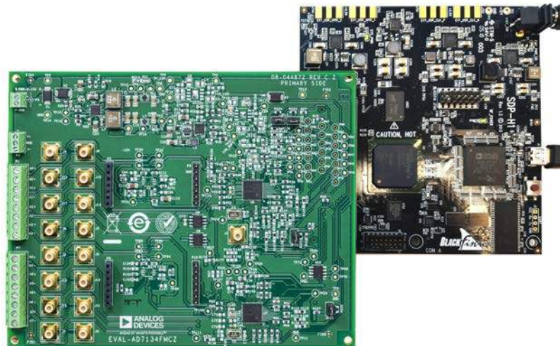
Figure 2. EVAL-AD7134FMCZ and SDP-H1 Board Connection
