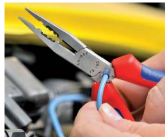
Crimping 20-14 AWG (0.5 to 2.5 mm 2 )
