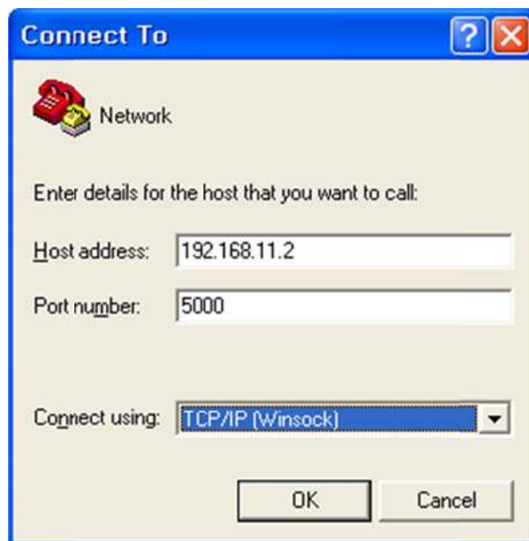
Figure 13. Network Terminal Program Configuration
