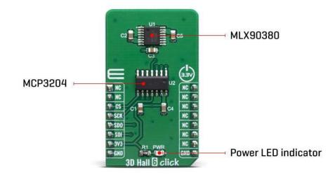
The magnetic sensor has a very low pin count. However, in order to allow reading of the 4 analog inputs on the single Click board<sup>™</sup>, 3D Hall 6 click have onboard 4-channel, 12-Bit A/D converter, with SPI interface. Thus, the communication interface procedure relies on reading the appropriate registers of the MCP3204.
