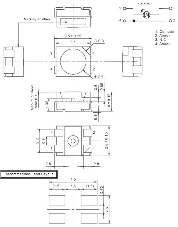
(Note1) Tolerance unless specified:  $\pm 0.1$  mm.
