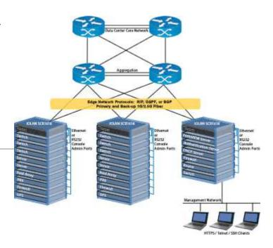
The **built-in firewall** offers intuitive policies to protect inside networks from unauthorized access. The firewall also allows inside networks to be separated from each other. If there are network resources that need to be available to an outside user, such as a web or FTP server, these resources can be placed on a separate network behind the firewall in a demilitarized zone (DMZ).
