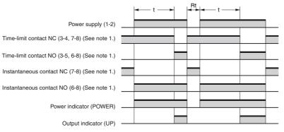
Note: 1. The R2 contacts (7-8 and 6-8) are programmable and can be set to either instantaneous or time-limit contacts using the switch located on the bottom of the Timer.
