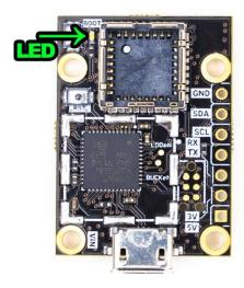
**LED:** When plugged in to micro-usb power and a Lepton is inserted in the socket LED will flash slowly. When video is being transmitted to the viewing program, LED will flash more rapidly.
