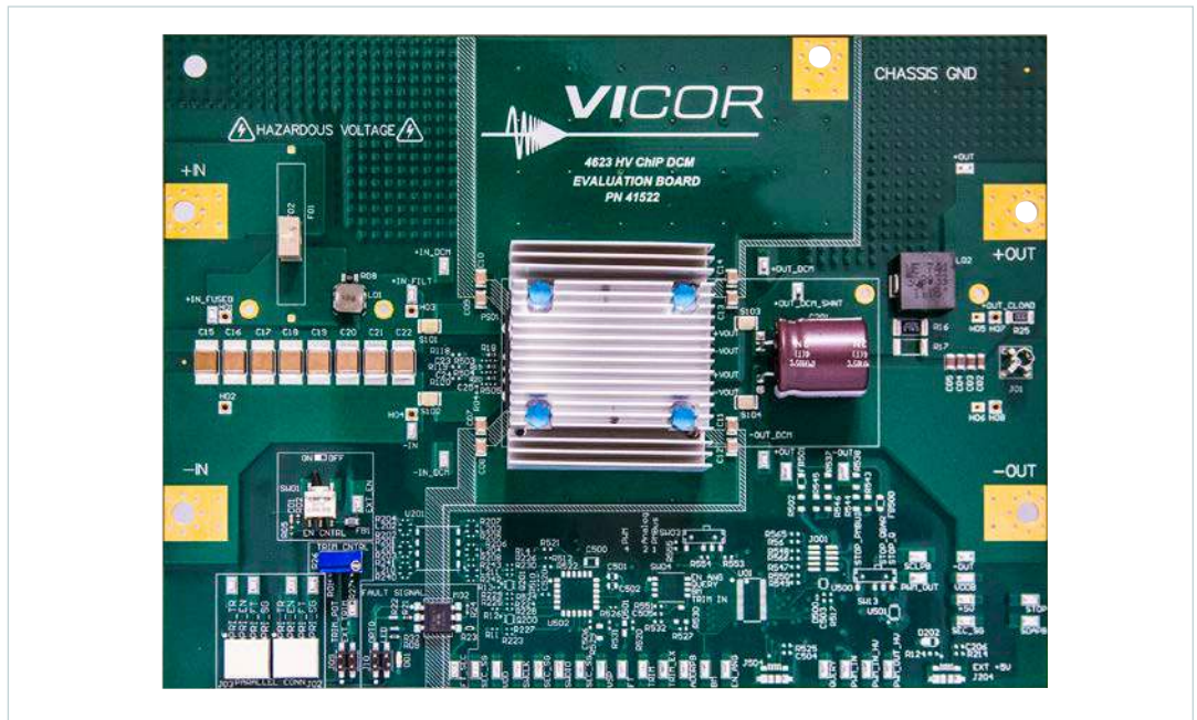
Figure 2 DCM4623 evaluation board photo, top side
