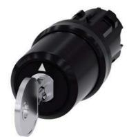
key-operated switch Siemens, 22 mm, round, plastic, lock number SSG10, with 2 keys, 3 switch positions I-O-II, latching, actuating angle 2x45°, 10:30h/12h/13:30h, key removal O+I, with laser labeling, upper case and lower case, always upper case at the beginning of the word
