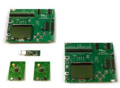
2 x SmartRF06 Evaluation Boards (SRF06EB) 2 x CC2538 Evaluation Modules (CC2538EM) 1 x CC2531 USB dongle (sniffer) 2 x Micro USB Cables Documentation
