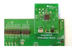
Insert a CC2538EM board into the SmartRF06EB as shown above. **NB! Note the jumper on the upper row on the header on the CC2538EM.**
