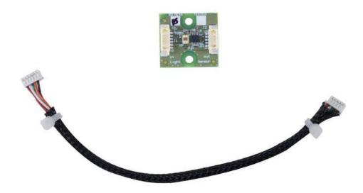
UDOO Bricks are modules you can use to augment your UDOO boards and make them more versatile. Attach them into I2C snap-in connector with the related cable. UDOO Bricks work along a cascade configuration, so you can attach them all together without wasting space in a truly intuitive way. Thanks to such configuration you can use cables up to 3,5 m long to connect UDOO Bricks one another.
