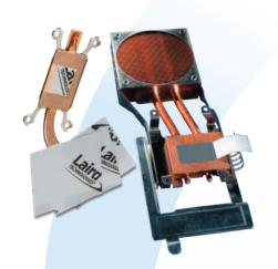
Tpcm<sup>™</sup> 900 is a high performance, non-electrically conductive phasechange material. At 50°C, Tpcm<sup>™</sup> 900 begins to soften and flow, filling the microscopic irregularities of both the thermal solution andthe component's surfaces, thereby reducing thermal resistance. It is a flexible solid at room temperature and freestandingwithout reinforcing components that reduce thermal performance.
