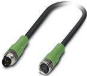
Sensor/Actuator cable, 4-position, PVC, Black RAL 9005, Plug straight M8, on Socket straight M8, Cable length: 2 m
