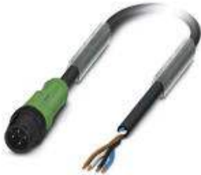
Sensor/Actuator cable, 4-position, PUR halogen-free, Black-gray RAL 7021, Plug straight M12, A-coded, on Free cable end, Cable length: 3 m, with plastic knurl
